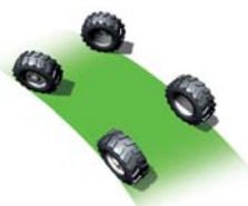
FRONT WHEEL STEERING MODE
